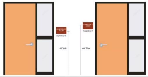
Place on latch side of a single door. If there is no space on the latch side, signs must be located on the nearest adjacent wall:
