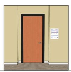
For double leaf doors with both sides active, the sign must be located to the right of the door. For doors with one active leaf, the sign must be located on the inactive leaf:
